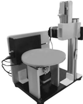
Figure 7 Example of the Automatic Glue Dispensing Tool for the Third Kaizen Improvement
