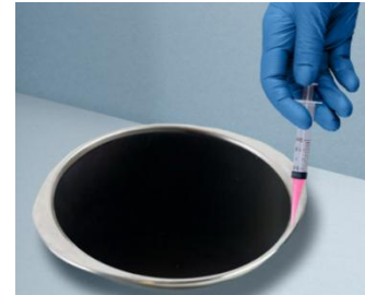
Figure 2 Example of Dispensing Adhesives around the Aluminum Tray
